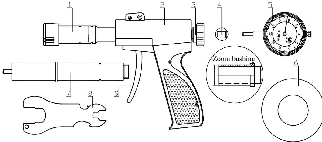
1. Measuring head    2. Pistol body    3. Locking nut    4. Bushing
